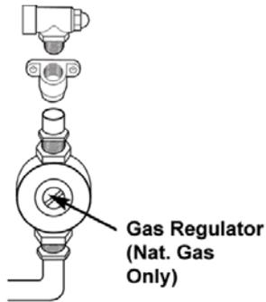
Connection to the gas supply should be made using the Aquaknect AS/NZS 1869 class B hose assembly with an internal diameter of not less than 10mm and regulator (regulator for use with natural gas)
